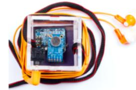
Figure 1: Low-cost hearing aid (LoCHAid). Sinha et al. PLOS ONE (2020)
